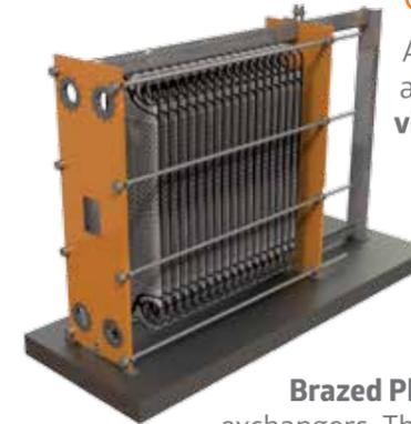
Braze Plate Heat Exchangers work on the same principle as the gasketed plate heat exchangers. The difference being that the heat transfer plates are brazed together. Resulting in a very compact heat exchanger.
