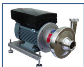
photo: KN3H Design KB pump on stainless steel machine feet with internal frequency converter max. flow rate: 50.000 l/h max. height: 48m @50Hz
