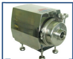
photo: KN2 Design A pump on stainless steel machine feet with stainless steel motor cover max. flow rate: 15.000 l/h max. height: 20m @50Hz
