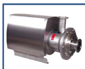
photo: S Design DV self-priming pump on stainless steel base with stainless steel motor cover max. flow rate: 40.000 l/h max. height: 28m @50Hz
